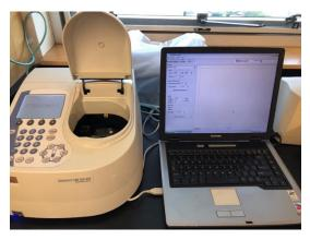
**<u>Results:</u>** My first completed graph of cyclic voltammetry, it didn't come out how we expected it to be. I would get different peaks in spots it wasn't suppose to be in. I realize after some long consideration, I didn't purge in enough nitrogen to remove the oxygen from the system. Once I purged in nitrogen for a significant amount of time, the graph came out to look like the one shown below.
