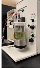
For our hypothesis, we used a spectroelectrochemical cell that is designed to monitor cell reactions spectrophotometrically (using UV-Vis instrument) while quantitative electron transfer is taking place at the platinum flag electrode. This set up was only tried once without putting the
