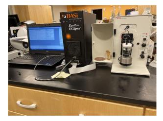
For cyclic voltammetry, I used this cell that has 3 electrodes. We use this cell to obtain a cyclic voltammetric plot to get different parameters. \_\_To set up a typical CV experiment, you have to purge inert nitrogen or any inert gas to keep oxygen at the bay throughout the operation using a two small tubes, one is to purge through the experimental solution and the other on is to be kept at the top of the solution to blanket the surface of the solution while CV measurement were been take.
