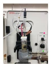
Once I couldn't get the cell going, I went back to the traditional way of spectroelectro chemistry and used a quartz cell that perfectly fits into the UV-VIS spectrophotometer.
