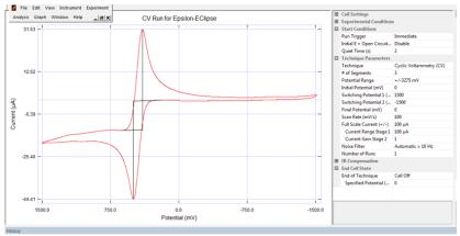
Once we started getting comfortable with the cyclic voltammetry technique, I used this plot and transferred some data into excel to do further investigation and retrieve a parameter. The parameter I was trying to obtain the diffusion coefficient in the Randles-Sevcik equation.
